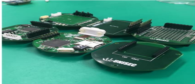
Figure 1. Six PCBs (one for each subsystem), with some electronics soldered on
