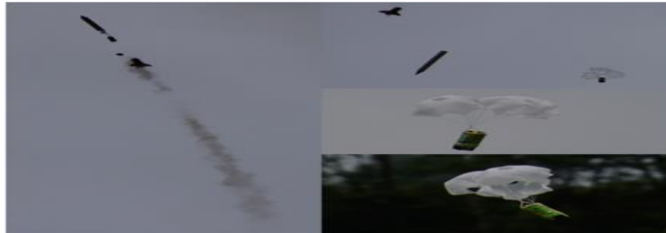
Figure 12. Separation from the rocket and successful parachute deployment.
