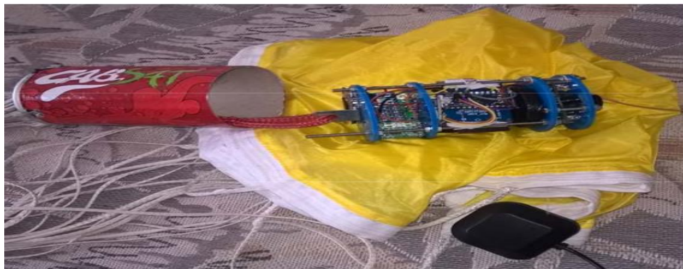
Fig. 3 – Pico-satellite embedded in the volume and shape of a standard soda can (height: 115 mm, diameter: 66 mm)
