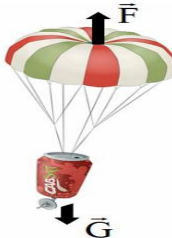
Fig. 8 – The structure of the CanSat parachute.
