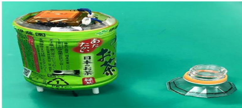
Fig. 3. Full system, introduced into a PET-bottle.
