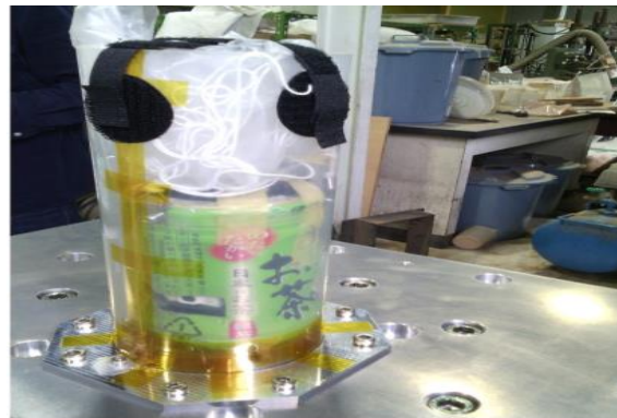
Fig. 6. Full system mounted in the setup for the vibration test.
