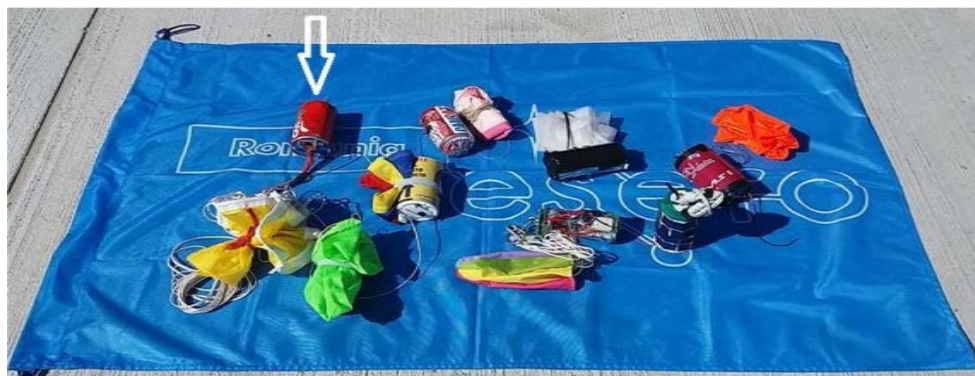
Fig. 3 – Pico-satellite embedded in the volume and shape of a standard soda can (height: 115 mm, diameter: 66 mm)
